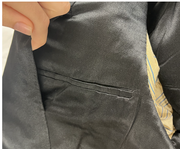
Fig. 9 The facing of the lapels is not secured over the interior lining.
